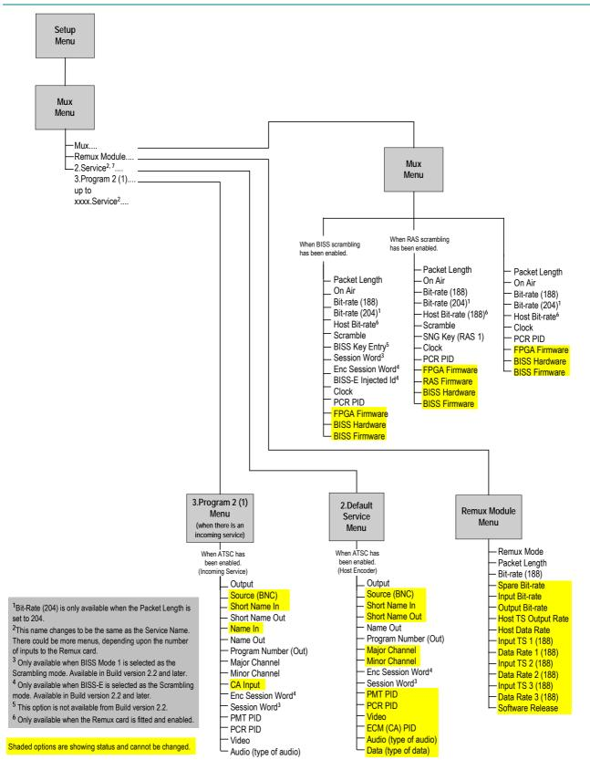
Figure 4.19: Menu Hierarchy – Setup/Mux Menu (ATSC)
